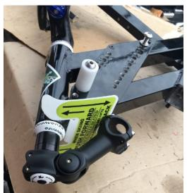
**#5** For shipping, the handle bar stem is rotated 180 degrees, lowered to a downward position, and the clamping screws retightened.
