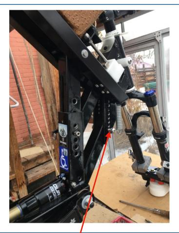
**#3** For shipping, the screws for attaching the bottom of the springs that raise the seat up for loading and unloading ski lifts are installed in the correct hole on the iSkibike.
