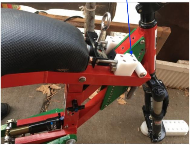
Sitting down on the seat with the back of the seat in the raised position, and with the push bars in the forward position, can bend the push bars. Make sure the push bar is moved to the position adjacent to the seat, before sitting down when the back of the seat in the raised position.
