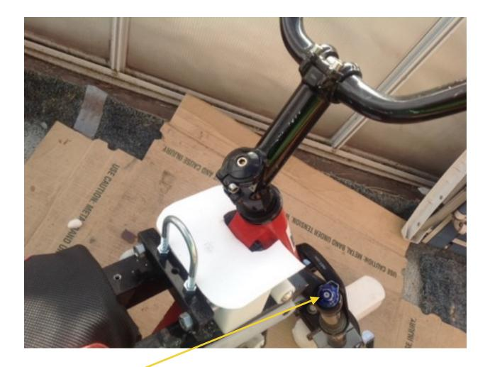
This blue knob on the fork labeled "Lockout" is used to disable the fork's suspension so a bicycle does not bob up and down from the force of peddling uphill. If for some reason a ski biker did not want front suspension, the lockout knob is rotated clockwise until it stops, as indicated by the directional arrow and labeling on the lockout knob.
