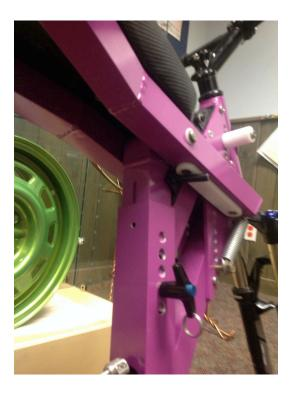
Here is the view of the seat blocker draw latch in the open position.
