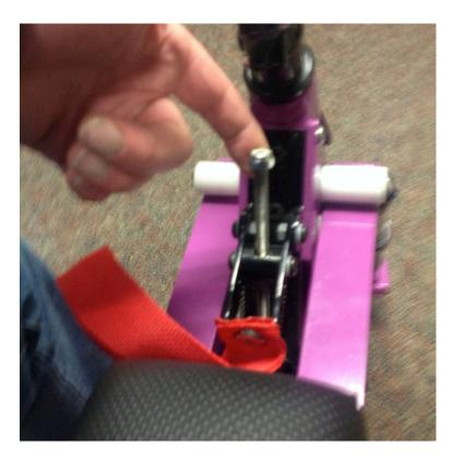
Top nut is now turned clockwise to tighten the seat blocker pull bar.
