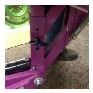
Seat blocker pull bar now does not contact under side of seat. It is too loose and needs adjustment.
