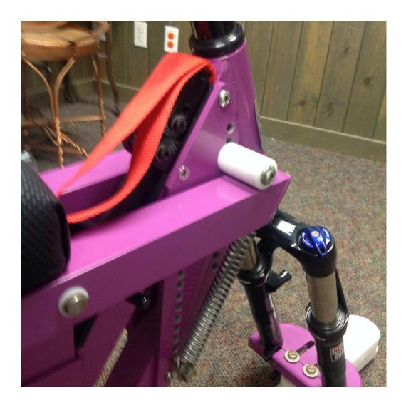
Please note that if the draw latch is inadvertently left closed and this is noticed while on the lift, The mechanism can be easily opened by pushing gently down on the handlebars while pulling the draw latch open. Once the draw latch is pulled open, the handlebars will spring back and up, so be prepared to control this motion.
