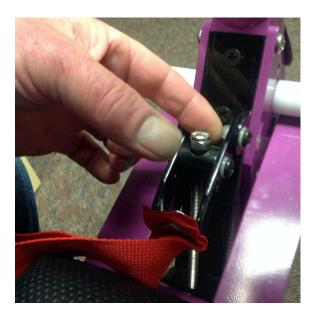
Seat blocker is properly adjusted when it snaps firmly into place, without needing more force than the rider can apply.
