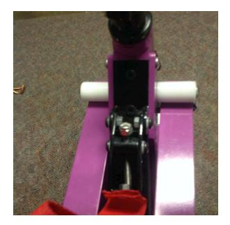
Sitting on the seat to hold it down in a riding position, As the seat blocker draw latch is closed, the pull bar hits the underside of the seat before the draw latch fully closes against the steering column. Thus the seat blocker needs adjustment. In this case loosening the pull bar by turning the top nut counterclockwise. Note the bottom wing nut inside the pull bar will not spin when the top nut is turned so it need not be held during adjustment.
