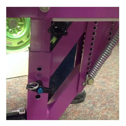
Extra length of adjustment rod sticking out shows seat blocker is loose and needs tightening.
